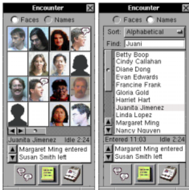
Figure 3. Design sketches of Encounter in the expanded state, used for large gatherings. Users can flip between the two views to see the faces of people viewing the same event or to view names and search for and sort them.
