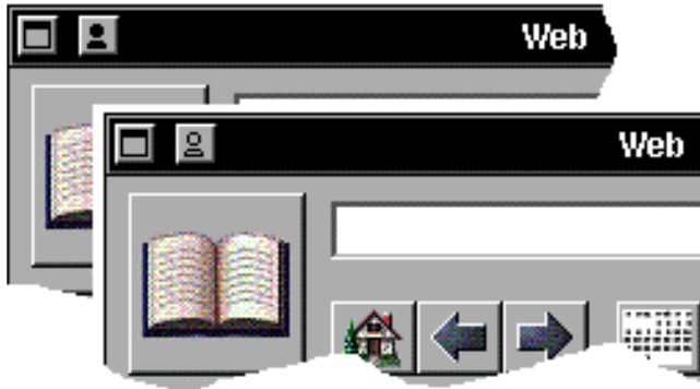
Figure 2. Design sketches of Encounter in the minimized state. The filled-in state indicates that others are nearby, the hollowed-out one shows that no one is nearby.
